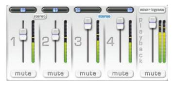
Pictured above is the INSPIRE 1394 Monitor Mixer, which is located within the Control Panel. This Monitor Mixer allows for flexible routing of your audio inputs before it reaches your software program. This is helpful in monitoring your live input without having to hear a delay resulting from the time it takes to process your audio in and out of the computer to your audio output device- called latency.
